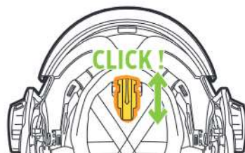
5 Adjust helmet incline angle for an optimum field of view
