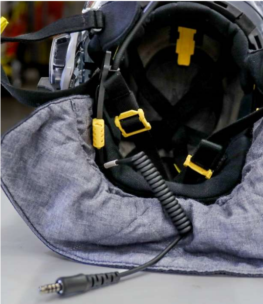
Figure 7: Yellow mount for Nexus plug
