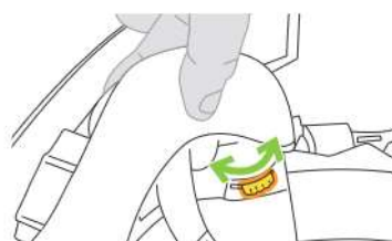
6 Adjust rear headband (x2) for neck comfort
