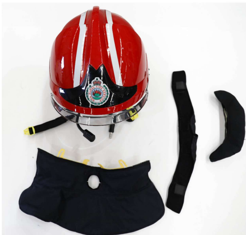
Figure 10: Soft components removed from helmet.
